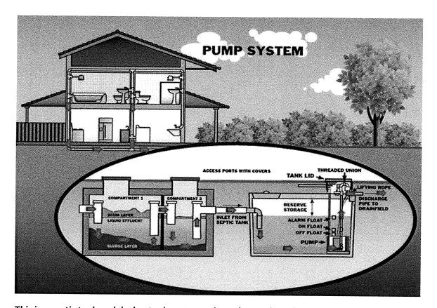
This is a septic tank and dosing tank system, where the septic tank is a two-compartment tank and the dosing tank houses a pump system.
