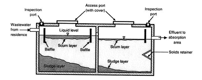
This is a standard, gravity-fed, two-compartment septic tank.
