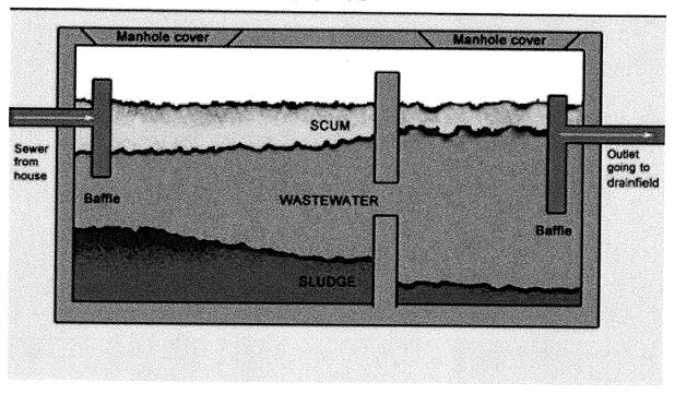
This is a standard, gravity-fed, single compartment septic tank.
