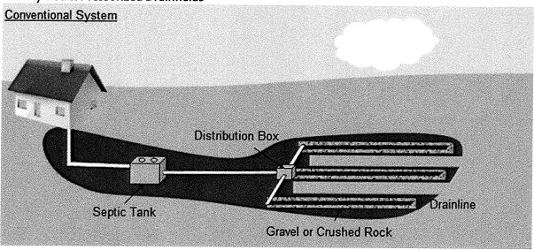
Most septic systems have the type of drainfield pictured above. It does not have a pump or any electrical components - instead the clear effluent flows using gravity only from the outlet side of the septic tank, to one or more distribution boxes.
