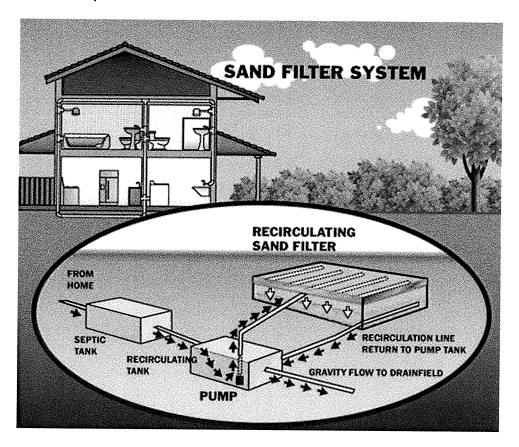
A sandfilter is one type of an Alternative Treatment Unit. These additional units are installed when either the lot is too small for a full sized drainfield, or the soil conditions are not ideal. These can be above ground, or they can be bottomless sandfilters below ground level. They allow for additional treatment of the effluent before it drains through the soil and into the groundwater, or occasionally the sandfilter will come before a small drainfield.
