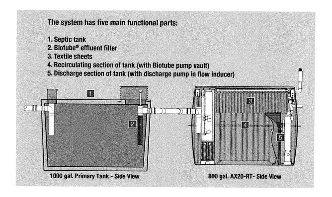
Pictured here is one common brand of an ATU or ATT, an Advantex AX-20 RT. These are now installed more often than a sandfilter, since they require less area to be used on the property and they clean the effluent much better. They are also less prone to failure overall. These ATU's are installed after the septic tank or the dosing tank and treat the effluent using either UV lights or additional filtration systems, then discharge the effluent to the drainfield.
